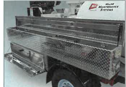
Expanded storage with locking diamond plate watertight job boxes for added security
